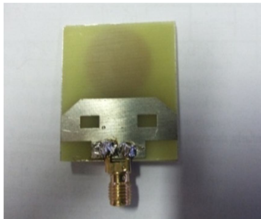
Fig.19.Fabricated ground plane view
