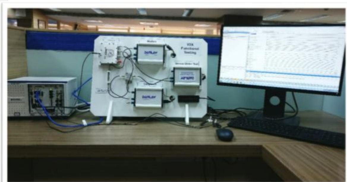
Figure 3: DANLAW HIL bench setup
