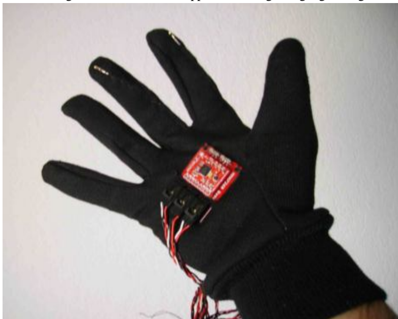
Fig. 3: Glove-based approach for sign language recognition [10]
