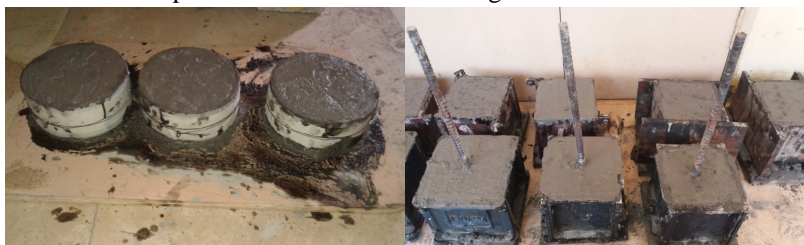
Fig. 4 Casting of Impact , Pullout and Cube specimen
