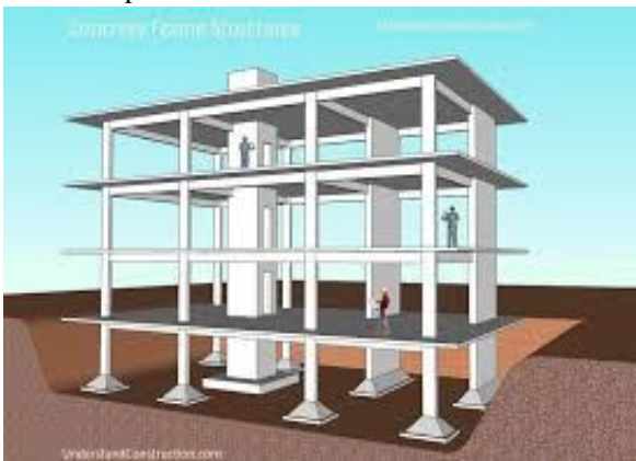
Fig. 1: RCC Frame structure
