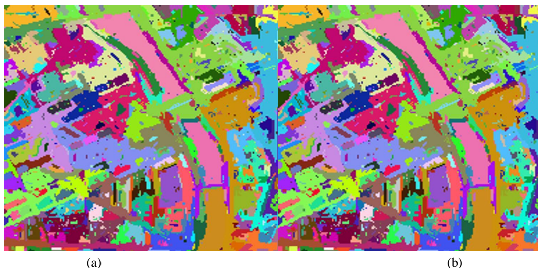
Fig.5. (a) segmented image obtained without image tiling (b) Segmented image after applying our tile-based region merging framework. No artifacts can be observed at the tile boundaries. Both results (a) and (b) have been compared with the Hoover metrics: RC = 1 . The equivalence of the result is proven.
