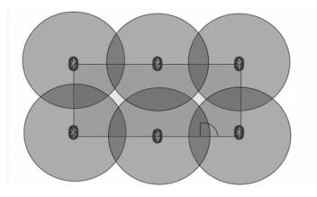
If placing beacons to a shop, then add one to the enrance of the shop. When a customer with a smart device installed on it enters/exits the shop, then the event will be triggered. If aiming for an accurate position in a building with multiple floors, it is recommended to add beacons right after the entering/exiting staircase or lift. The places where you do not want an accurate position, leave it with less number of beacons [8].
