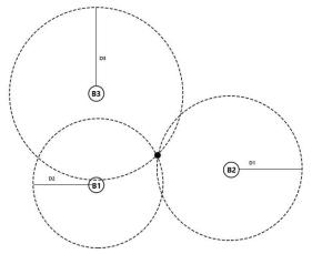
By measuring the distance of the known anchors, it is possible to know the required point's position. If we measure a certain distance, then we will be in a circle of that radius around the anchor. By measuring the distance with three anchors, it seen that the position is uniquely determined by the intersection of the three circles. This method is known as Trilateration. The circles do not always intersect at exactly one point. Therefore, we try to find the point closest to all the circles
