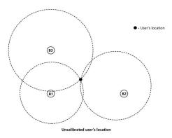
Initially, the AR device needs to be calibrated in order to determine the initial location from where we can start tracking. As the location data provided by the Bluetooth beacons will just be in respect to them, we need to relate it to the real world in order to start using it in AR scene. Further on, we can use the initial location as a reference in order to pinpoint location of a user. For calibration, the devices use its camera as an input in order to determine user's current location.
