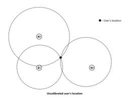
Initially, the AR device needs to be calibrated in order to determine the initial location from where we can start tracking. As the location data provided by the Bluetooth beacons will just be in respect to them, we need to relate it to the real world in order to start using it in AR scene. Further on, we can use the initial location as a reference in order to pinpoint location of a user. For calibration, the devices use its camera as an input in order to determine user's current location.
