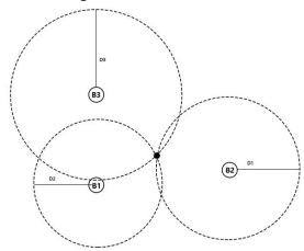
By measuring the distance of the known anchors, it is possible to know the required point's position. If we measure a certain distance, then we will be in a circle of that radius around the anchor. By measuring the distance with three anchors, it seen that the position is uniquely determined by the intersection of the three circles. This method is known as Trilateration.
