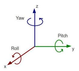
Angle of x axis is known as Roll Angle of y axis is known as Pitch Angle of z axis is known as Yaw
