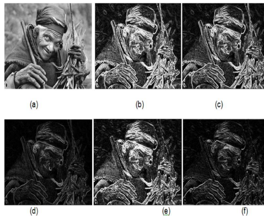
Figure. 13 Comparison of Edge Detection Techniques (a)Original Image (b) Sobel (c) Prewitt (d) Robert (e) Laplacian (f)Laplacian of Gaussian.
