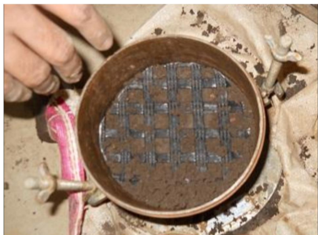
Fig:2 Geogrid material placed into CBR mould
