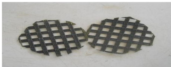
Fig: 1 Geogrid material cut in circular disc for placing in CBR mould
