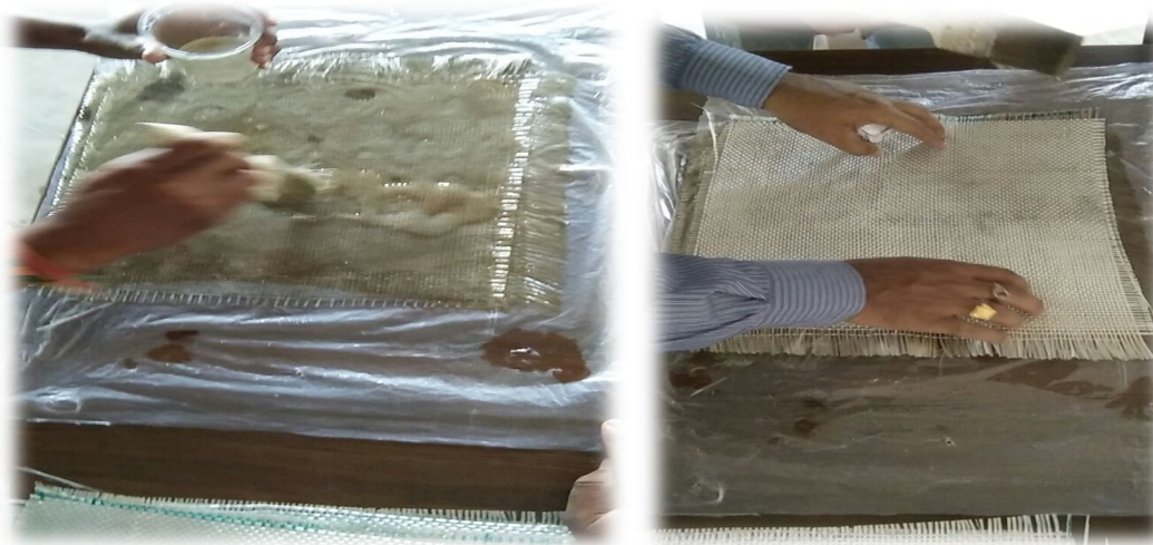
Fig11: Sample preparation by wet hand lay-up process
