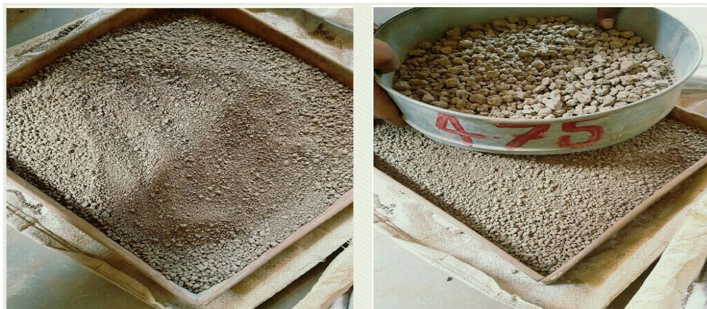
Fig.1.Blackcotton soil after oven dring
