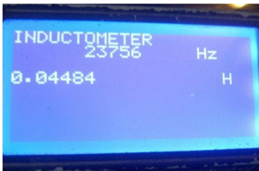
Fig.14 Result of a tested inductor
