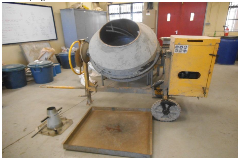
Fig 4 Drum mixer used for mixing concrete in laboratory
