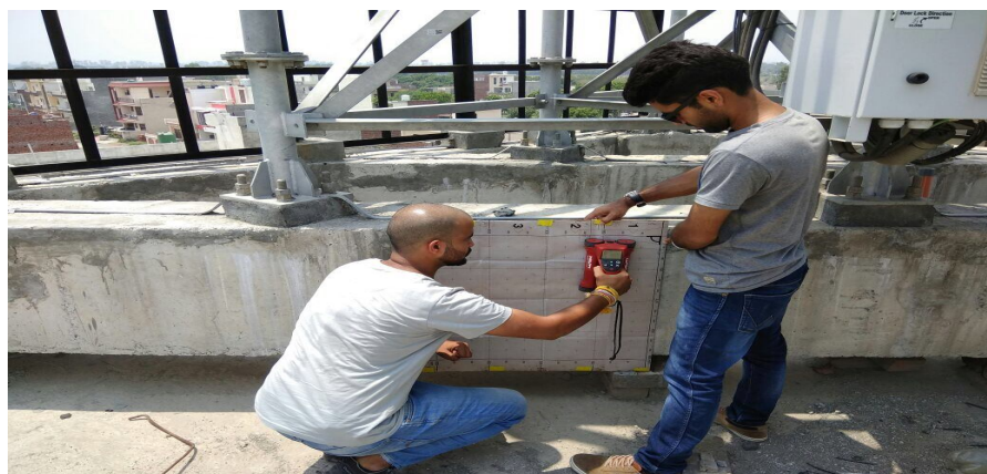
Figure 6 Conducting Ferro scanning of Beam 4
