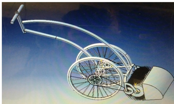
Fig.1 Design of Eco Friendly road cleaning machine
