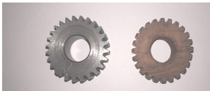
Fig. 14 Gear Cut using the Attachment
