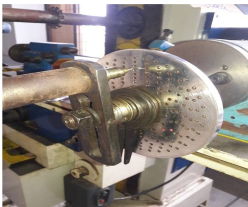
Fig. 11 Indexing Plate and Indexing Pin
