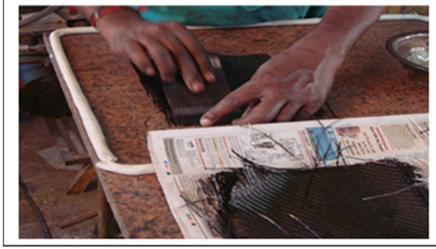
Fig 1: Hand lay up technique- Carbon Laminate
