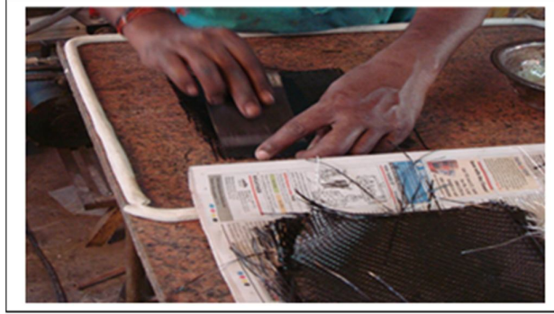
Fig 1: Hand lay up technique- Carbon Laminate
