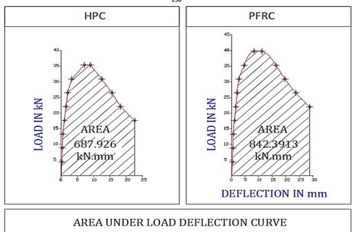
The flexural toughness factor for High Performance Concrete was found to be  $9.5545 \times 10^{-3}$  and that of Fiber reinforced High Performance Concrete was found to be  $11.79 \times 10^{-3}$ . There was an appreciable increase in the flexural toughness factor by the addition of fiber in HPC.
