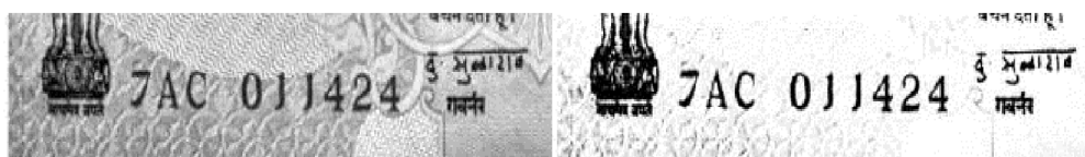
Figure 4.6.2. Edge based segmentation of serial number
