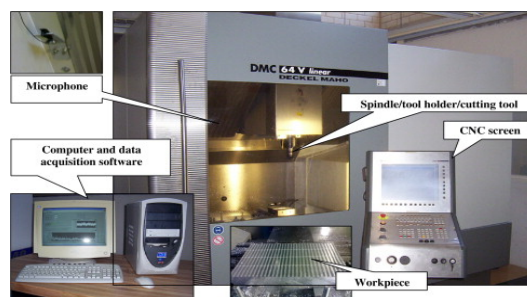
Figure 2. Experimental setup for finding stability lobe diagram. [8]
