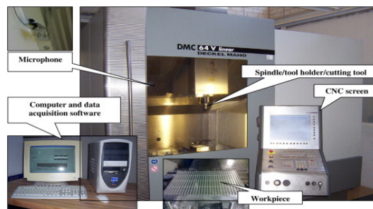
Figure 2. Experimental setup for finding stability lobe diagram. [8]
