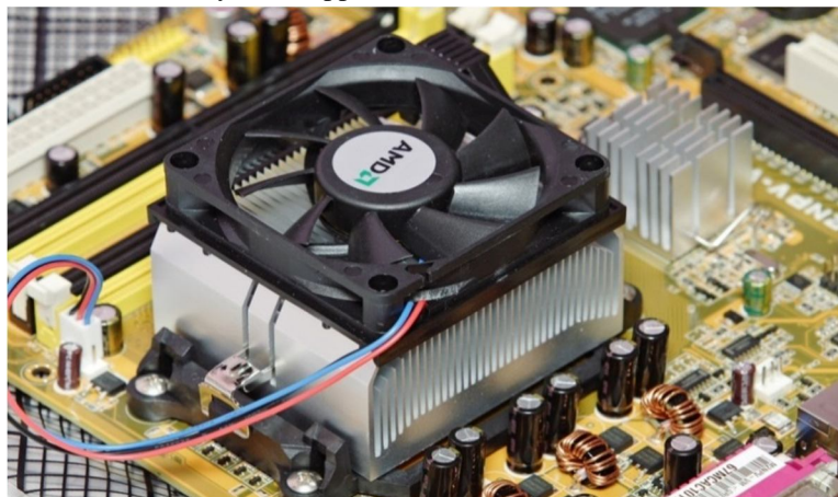
Fig. 2: A fan-cooled heat sink on the processor of a personal computer. To the right is a smaller heat sink cooling another integrated circuit of the motherboard.
