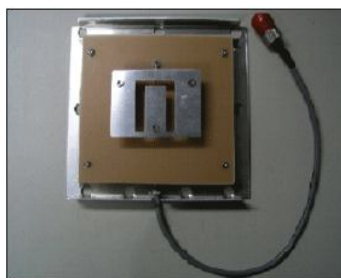
Fig.2. practical U-slot patch antenna
