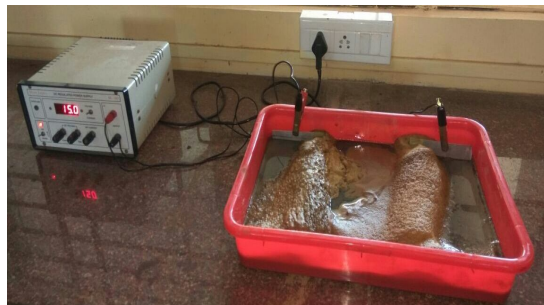
Fig: 4 image of electro coagulation reactor
