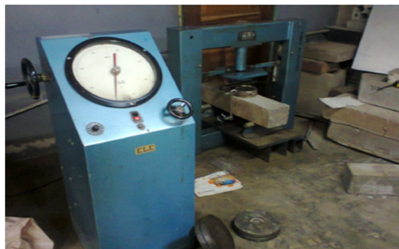
Fig:2 Testing machine U.T.M.
