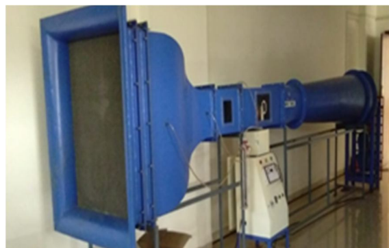
Fig 21: Wind Tunnel Test Setup from Outlet Side
