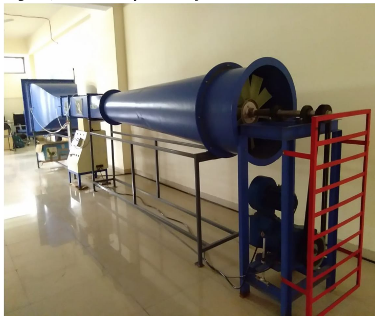
Fig 20. Wind Tunnel Test Setup from Inlet Side
