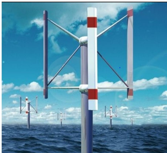
Fig.2. Vertical Axis Wind Turbine ( VAWT )
