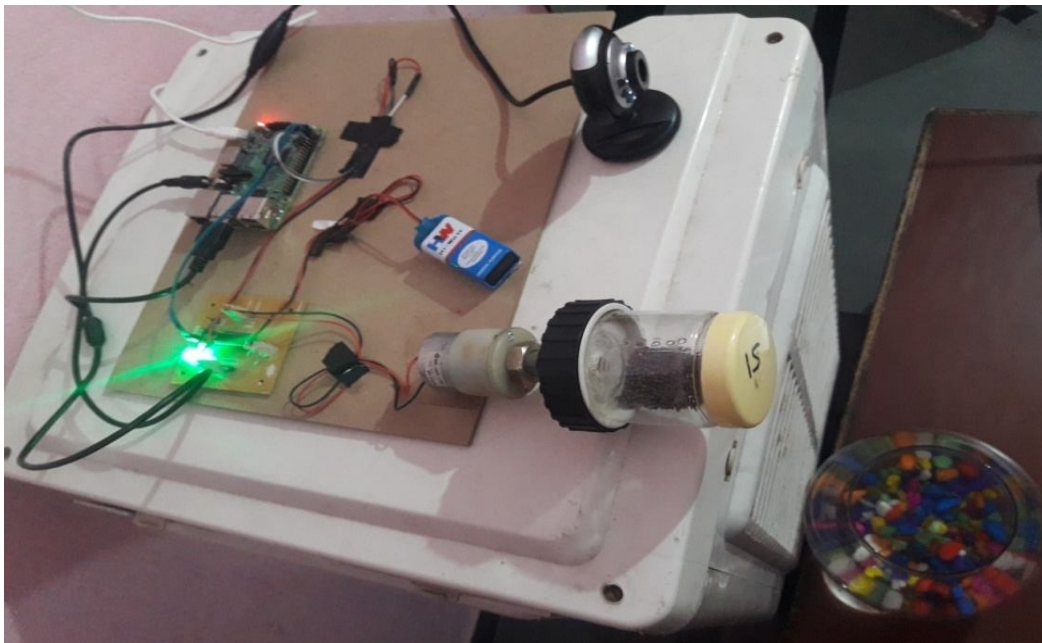
Fig. 2 Experimental setup of Automatic controlling of fish feeding system
