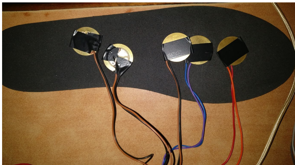
Fig.3 Array of piezoelectric sensor
