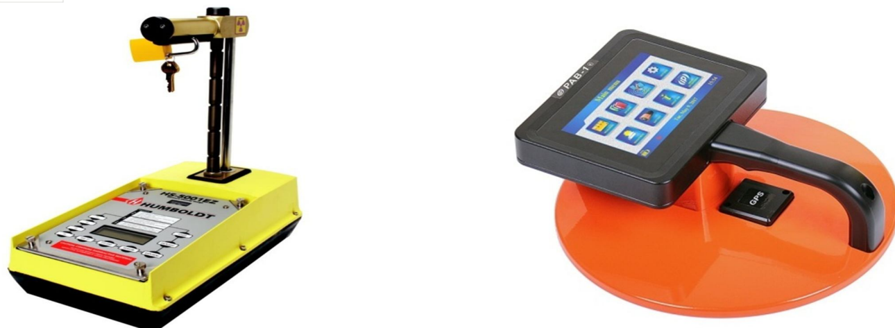
Fig. 1 Nuclear density gauge and non-nuclear density gauge
