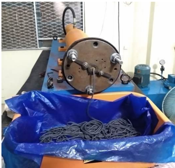
Figure 4.5: Abrasive media extruded through specimen
