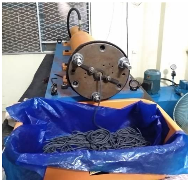
Figure 4.5: Abrasive media extruded through specimen
