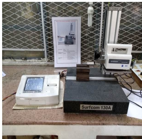
Figure 4.6: Surface roughness measuring instrument (Surfcom 130A)
