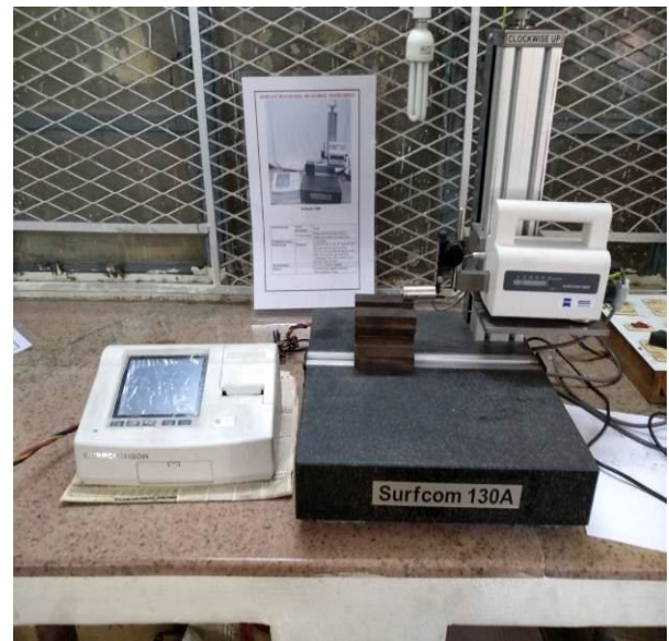
Figure 4.6: Surface roughness measuring instrument (Surfcom 130A)
