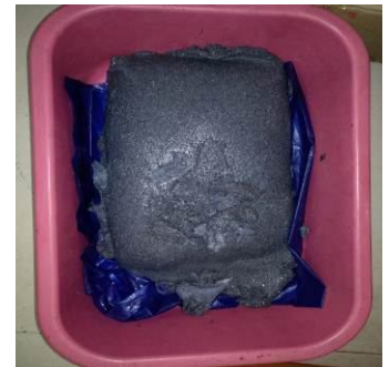
Figure 4.4: Silicon polymer with abrasive
