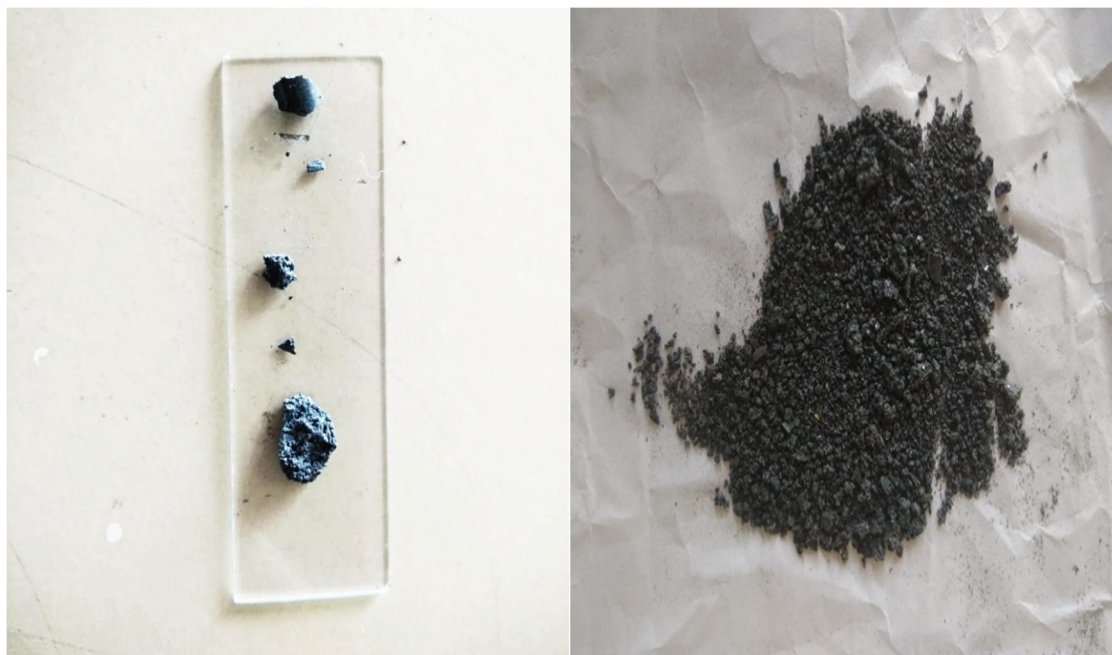
Fig. 2 Grown Crystals using Zone Leveling Method
