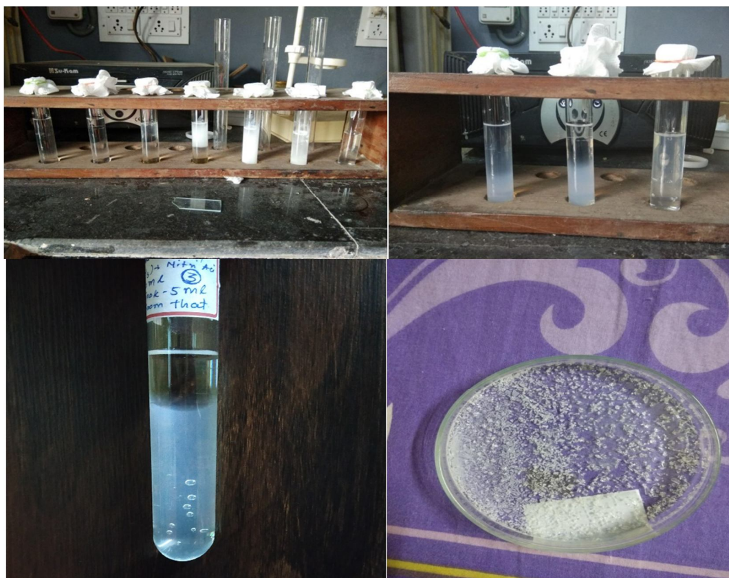
Fig.3 Gel Method and Grown Crystals
