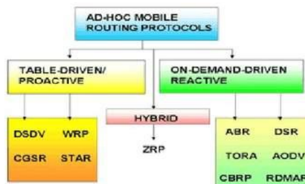
Figure 1: Classifications of routing protocols
