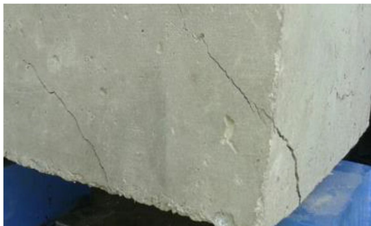
Fig .2 Cracks in bubble slab
