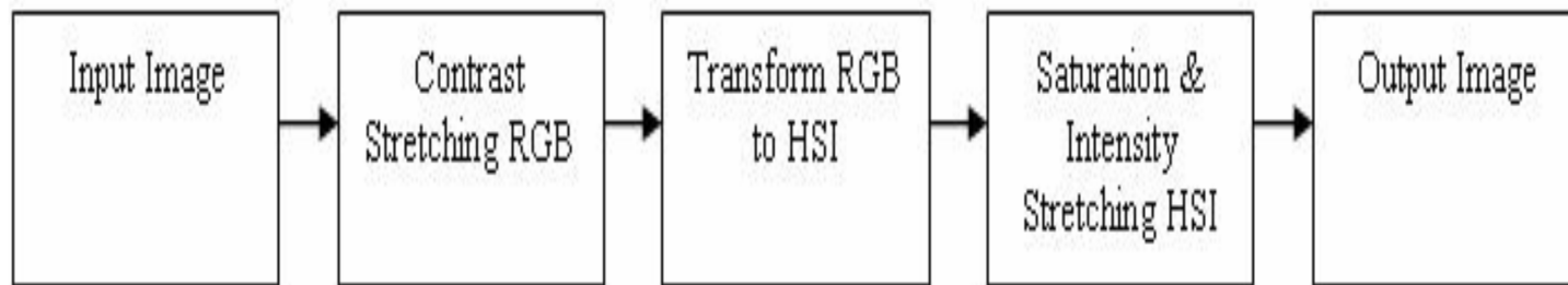
Figure 3: Our proposed Methodology for Underwater Image Enhancement
