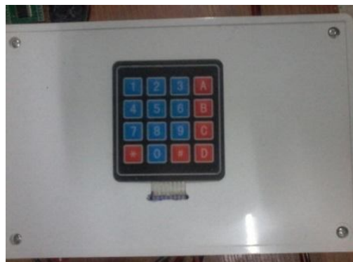
Fig. 7 The Circuit Casing showing the Keypad
