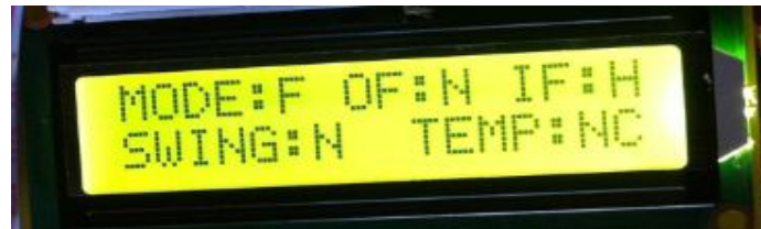
Fig. 8 LCD Display for Fan Mode of the RF Remote Control
