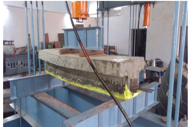
Fig 6:- Deflected shape of Post Tensioned Beam
