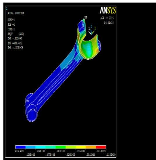
Figure 12 :Von-Misses Stress Output of the Stainless Steel Connecting Rod
