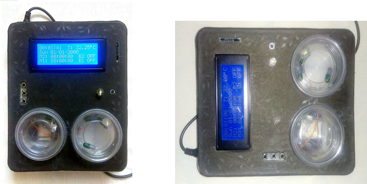
Fig. 2 Hardware model of medicine box
