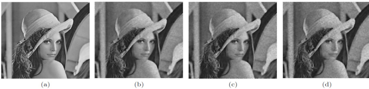
Figure 6: (a) Original image, 512 by 512, 8bits/pixel, with MSE = 0, PSNR = 1, (b) Restored image of noise var.0.04,(c)Restored image of noise var. 0.06, (d) Restored image of noise var.0.08
