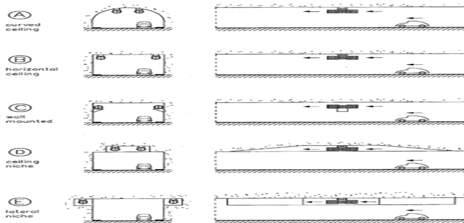
Typical Jet Fan Installations in road Tunnel
