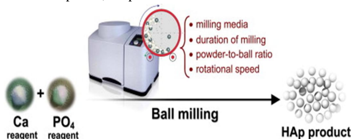
Fig. 2 Preparation of HAp nanoparticles via mechanochemical method.
