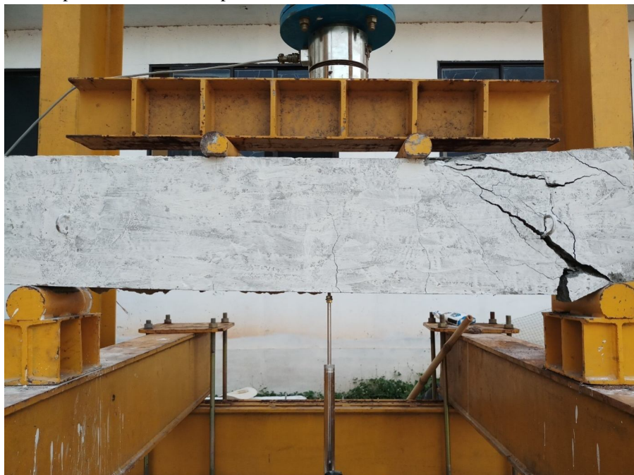
Fig. 17 Development of cracks in RCA25MS8 specimen
