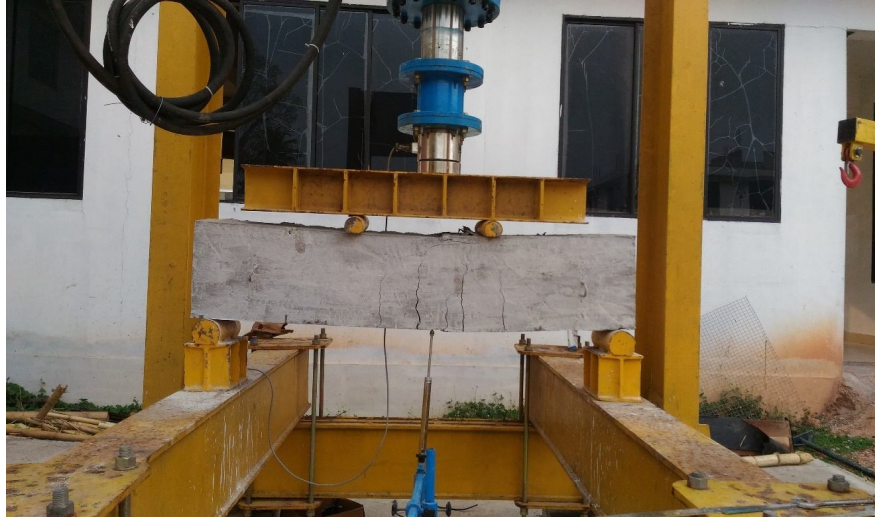
Fig. 16 Development of cracks in control specimen
