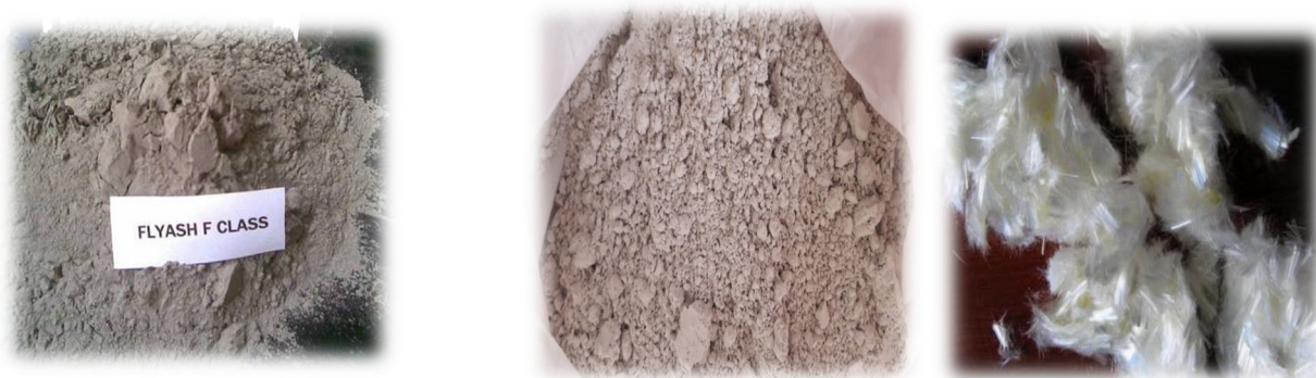
Figure 1: fly ash and Alccofine 1203 , PVA fiber
