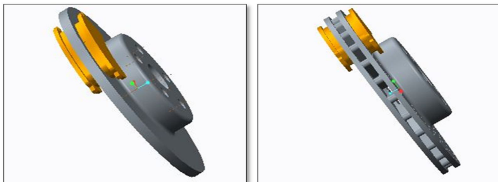
Fig 2: 3D- models of solid and ventilated disc brakes
