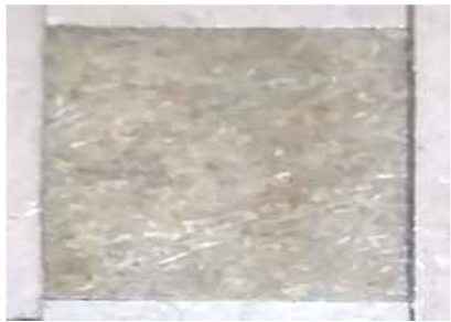
Fig. 5 Mould filled with Epoxy resin and reinforcement
