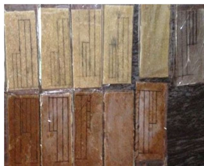
Fig. 6 Composites prepared and marked for cutting
