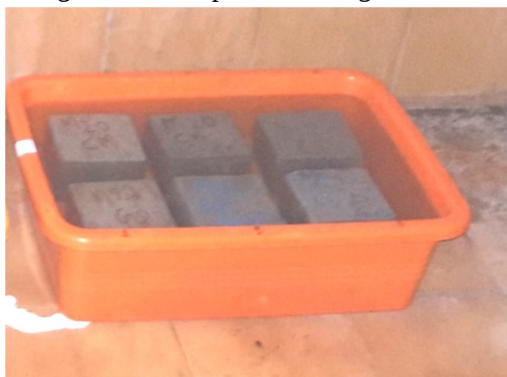
Figure V Specimens Immersed in MgSO_4 with Na_2SO_4 Solution
