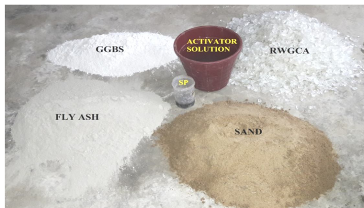
Figure III Materials used for RWGCA Geopolymer Concrete
