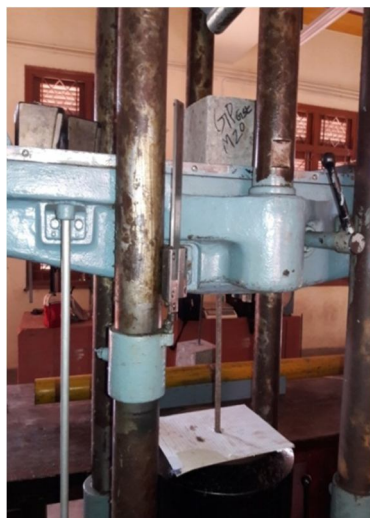
Figure VIII Pull Out Test Set up (RWGCA Specimen)
