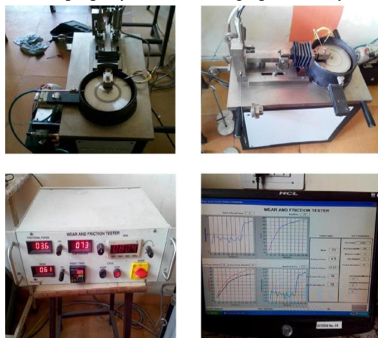
Figure3.9: Wear Tester Machine
