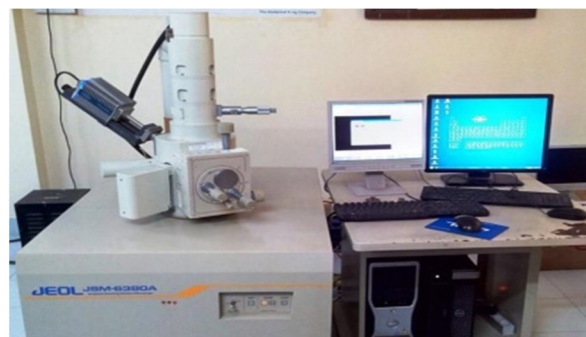
Figure 3.6: JEOLJSM-6380A SEM Instrument
