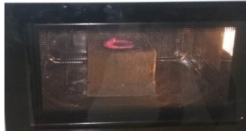
Figure 3.4: Microwave Experimental setup showing cladding process
