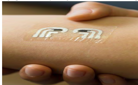
Fig. 3: Tattoo based Glucose Monitoring
