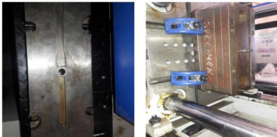
Fig 4.6 (b) Molds used in injection molding
