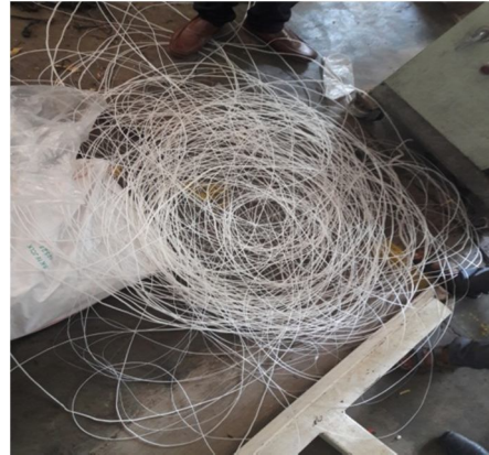
Fig 4.4 Product formed after Twin-Screw Extruder.
