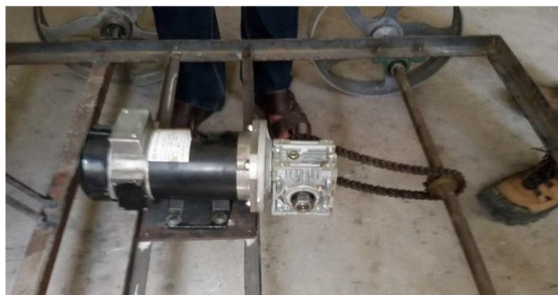
Fig 10. Setup of Motor and Chain Drive
