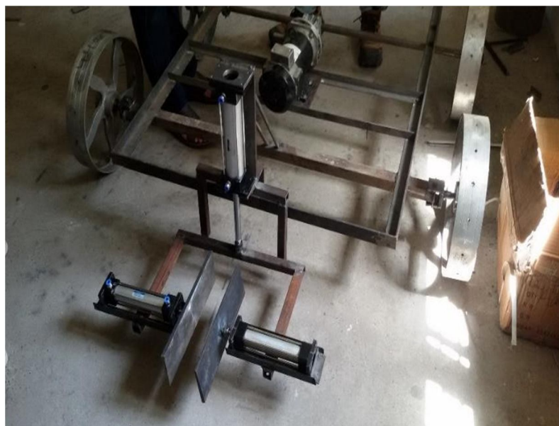
Fig 9. Arrangement of Pneumatic Cylinders
