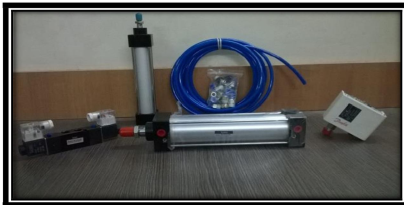
Fig 7. DCV, Cylinders, Pressure switch and pipe etc
