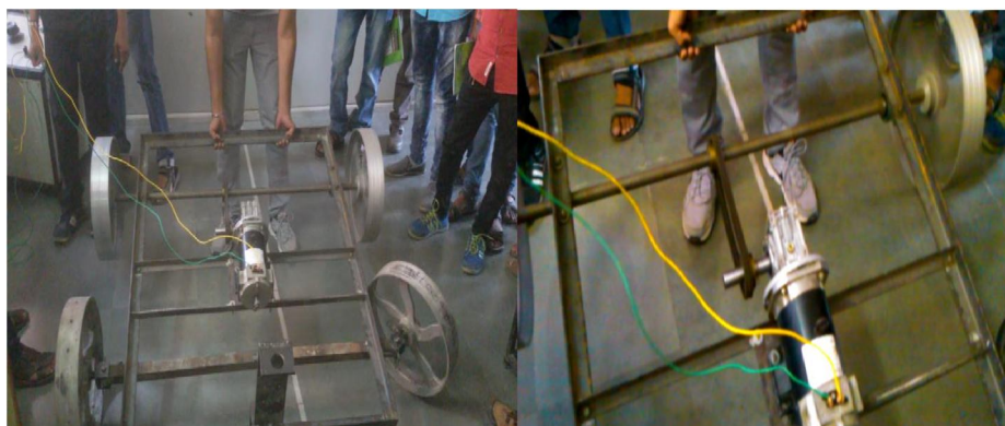
Fig 13. Traction system of AgriBOT
